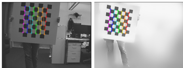
Figure 10. Calibration. Frames from the standard FLIR camera (top) and grayscale frames reconstructed from events (bottom), both with checkerboard corners used during calibration.
