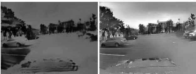
Figure 12. Reconstruction from (i) a network trained only on real event data from the DAVIS240C sensor (left), and (ii) a network trained only on simulated event data (right). This sequence is from the MVSEC dataset, and was recorded with a mDAVIS346 sensor.
