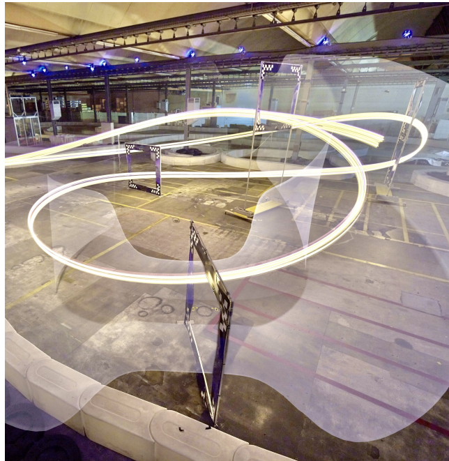
Fig. 1: Long exposure picture of our quadrotor flying at more than 80km/h in a physical racing track. The safety set is shown in translucent white, expanding in gate-free regions and constricting at gate passages. The safety set is a crucial element of our approach, thanks to which we can consistently prevent gate collisions and achieve 100% success rate in real-world experiments, even when operating at the drone’s physical limits.
