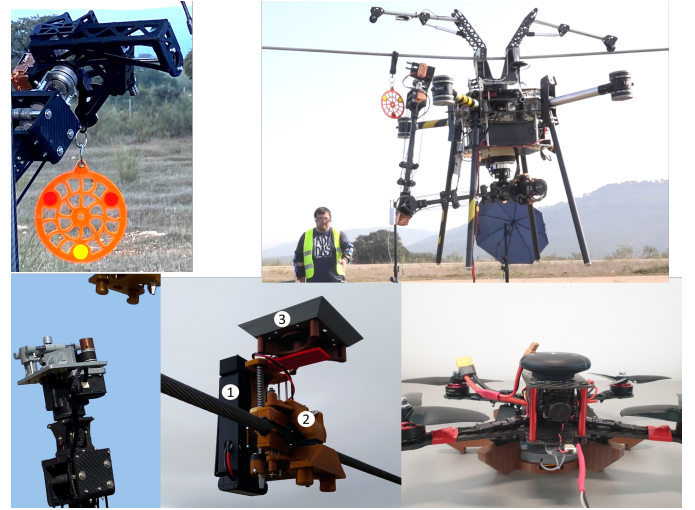
Fig. 7. (Top) Left: Clip-type bird diverter end-effector. Right: Installation of clip-type bird diverter with IMU-based teleoperation method. (Bottom) Left: Small recharging station end-effector. Middle: The fully integrated system of the lightweight charging station (1 - the electronics compartment; 2 - split-core current transformer; 3 - V-shaped landing station). Right: The fully integrated system of the drone HolyBro QAV250 and the receiver assembly.
