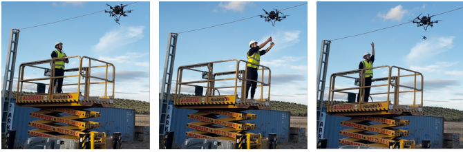
Fig. 9. Tool delivery demonstration. (Left) The gesture “palms together” causes the pulley to descend. (Middle) The operator retrieves the tool. (Right) The gesture “arm up” commands the pulley to rise.
