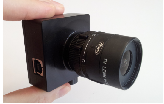
(a) The Dynamic Vision Sensor (DVS).
