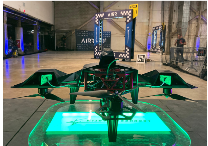
Fig. 1. Our AlphaPilot drone waiting on the start podium to autonomously race through the gates ahead.
